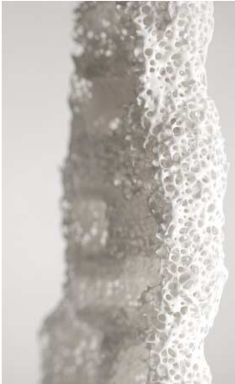
52 Ecorché structurel. Frittage par laser. SLS. 1/100° Structural cutaway. Model by laser sintering.
