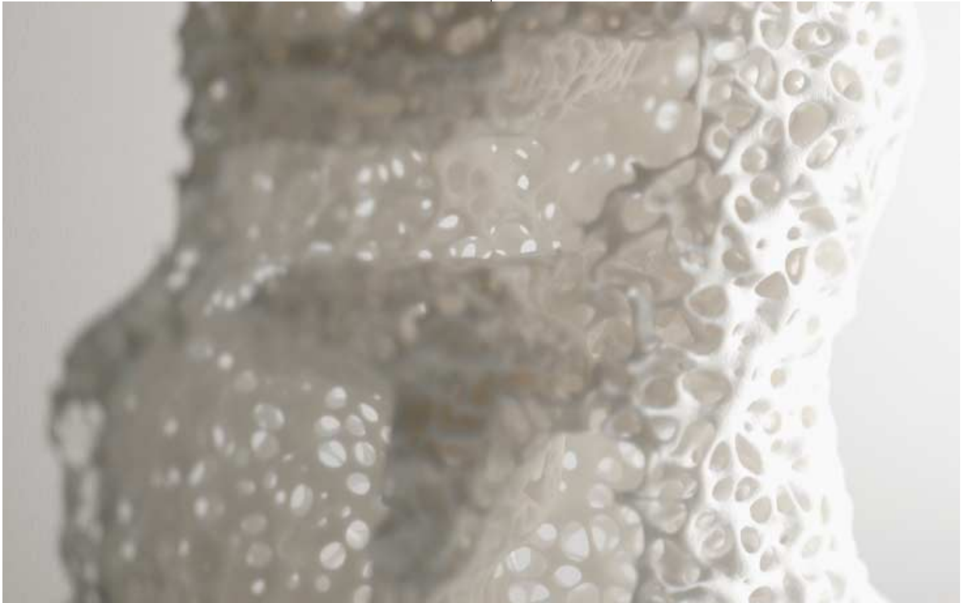
42 Ecorché structurel. Frittage par laser. SLS. 1/100' Structural cutaway. Model by laser sintering.
